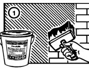
Then immediately rub KÖSTER KD 2 Powder into the fresh, moist slurry by hand until the surface is dry.
